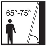
The correct erection angle for the ladder is 65-75°
