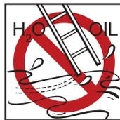
Ensure ground is free from contaminants. LADder must not be erected on a wet or slippery base.
