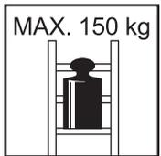
Max. load for the ladder is 150 kg.
