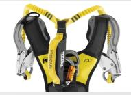
The harnesses have a parking system for the MGO connectors on fall-arrest lanyards on each shoulder strap. In the event of a fall, the system releases the MGO connectors and allows the absorber to be deployed.
