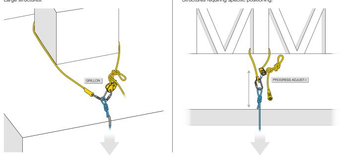
Temporary anchors with multiple configurations.
