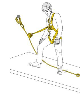
Kit for protection against falls, with NEWTON harness and ASAP LOCK mobile fall arrester ASAP LOCK FALL ARREST KIT is a ready-to-use kit designed to protect against falls from height. It contains a NEWTON fall-arrest harness, an ASAP LOCK mobile fall arrester with locking function, an ASAP'SORBER energy absorber, two OK TRIACT-LOCK carabiners, an ANNEAU open loop sling, an AXIS 11 mm rope with sewn termination, a weight, and a BUCKET bag. The kit is available in two sizes and two lengths.
