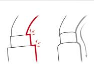
Fluid interior design Fluid interior design limits the risk of having a catch point and facilitates rotation of the carabiner.
