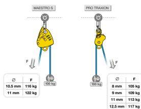
Here are some test results using a constant rate of 1.5 m/minute. Other results are available in the technical information at www.petzl.com
