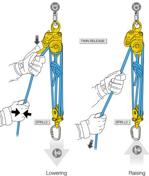
• Disadvantage: rigging is required to transition between lowering and raising
