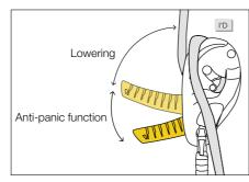
Designed for work at height, rope access, and technical rescue and evacuation, these devices are equipped with an anti-panic function and an anti-error catch, to reduce the risk of an accident due to user error. They are also compatible with auxiliary brakes, which help increase the friction for lowering heavy loads.
