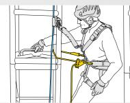
The GRILLON lanyard can be used in double mode (on the harness side attachment points) when the user works with weight on their feet. This type of attachment provides better load distribution on the belt. The user precisely adjusts their position by pressing on the lanyard's pivoting cam.
