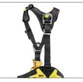
ASTRO BOD FAST full-body harnesses are equipped with a dorsal attachment point for attaching a fall-arrest system. In the event of a fall on this attachment point, a shorter adjustment of the length between the waistbelt and the leg loops means the load is taken up on the leg loops, allowing the user to remain suspended longer while awaiting rescue.
