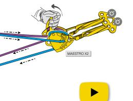
How to belay with the MAESTRO on a back-up rope
