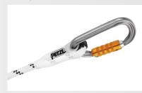
Sewn terminations with plastic sheaths Sewn terminations increase strength (compared to a knotted termination) while reducing bulk. These plastic sheaths protect the stitching from abrasion and facilitate handling by holding the connector in position.
