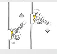
Integrated locking In the event of a sudden movement due to a fall, slide, or uncontrolled descent, the ASAP and ASAP LOCK mobile fall arresters lock on the rope and stop the worker's fall, even if they grab the device with their hands.
