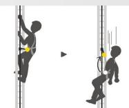
Ventral attachment point suitable for vertical progression on a rail or cable The LADDER CLIMB attachment point allows for ventral attachment of the fallarrest trolley, which distributes the load on the waistbelt, providing optimal comfort. In the event of a fall, the attachment point automatically moves upward to a sternal position to help keep the body in a vertical post-fall position (only on European versions).
