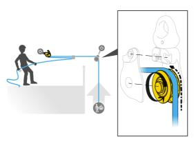
Extra friction makes for a more comfortable descent: the sheave does not rotate, and the facets provide additional friction on the rope.
