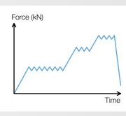
In the event of a fall, the tearing of the energy absorber webbing limits the impact force on the user. The lanyards are designed for users who weigh between 50 and 130 kg. The progressive tearing of the webbing reduces the deceleration on lightweight users
