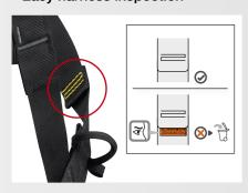
The sternal and dorsal attachment points are equipped with visual indicators: a red tag appears after a fall to indicate that the harness must be retired.
