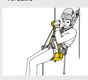
Self-braking descenders are versatile and can be used for both descents and short rope ascents.
