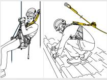
Effective in many different situations These mobile fall arresters work equally well on vertical or angled ropes, to adapt to a variety of different worksite situations.
