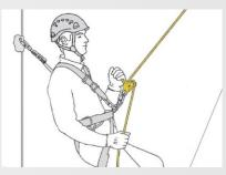
Single mode use When the anchor is located above the user, the GRILLON lanyard is connected to the harness ventral attachment point, so that the load is comfortably distributed between the waistbelt and leg loops. The user adjusts their position by operating the handle, while holding the free end of the lanyard.
