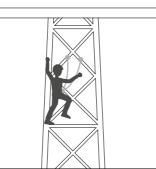
The ABSORBICA-Y lanyards with two arms allow for continuous protection by successively detaching and re-attaching the two arms
