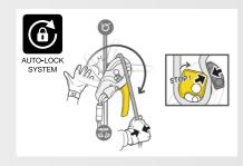
AUTO-LOCK system The AUTO-LOCK system allows users to easily position themselves at a workstation without having to manipulate the handle or tie off the device: as soon as the user releases the handle, the rope is automatically locked in the device.
