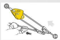
The integrated progress-capture pulley with very large diameter sheave mounted on sealed ball bearings rotates in only one direction for excellent hauling efficiency. The lower connection point can be used to create different types of haul systems.
